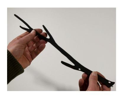
1. Remove all the sharp edges from the top and bottom with a pair of pliers, file and abrasive paper.
