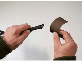
2. The smooth side of the leather is the upper side. Thread the leather lace through a hole in the twig. Leave approximately 10 cm protruding. Lay this 10cm flat on the steel. This will cause the leather to bulge up and this makes it more pleasant to hold.
